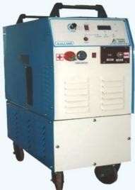
With the help of oil free compressed air delivery at 5.5 kg/cm<sup>2</sup> and electricity cut all metals like Stainless Steel, Mild Steel, Copper, Brass, Aluminum, Inconel, Monel, Titanium, Nickel, Chrome, Bronze, Galvanized Steel, Heated Steel, Wear Plates etc.
